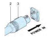
Connect the cable socket (2) to the chassis plug (1) and turn the socket clockwise by 45 degree to fix it.
