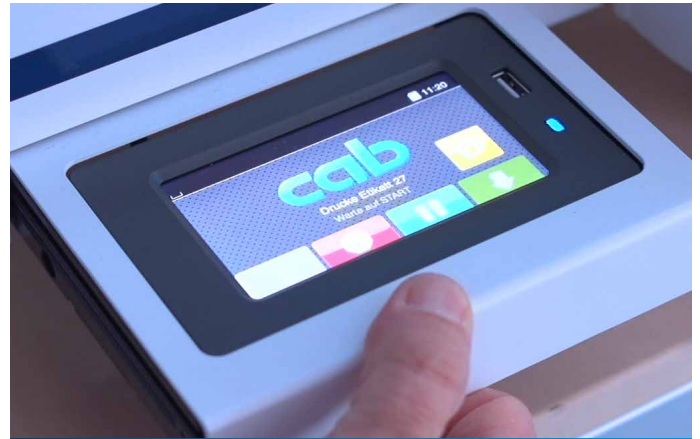
External cab control panel, touch function, integrated to a X-TubeProcessor casing
