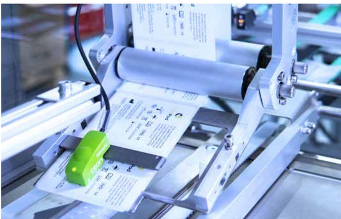
To detect even smallest differences in height in moving material webs, the CEON sensor can be assembled to the peel-off plate of IXOR. This prevents negative influences from stretching materials. Each label to peel off next by the IXOR plate can be verified.
