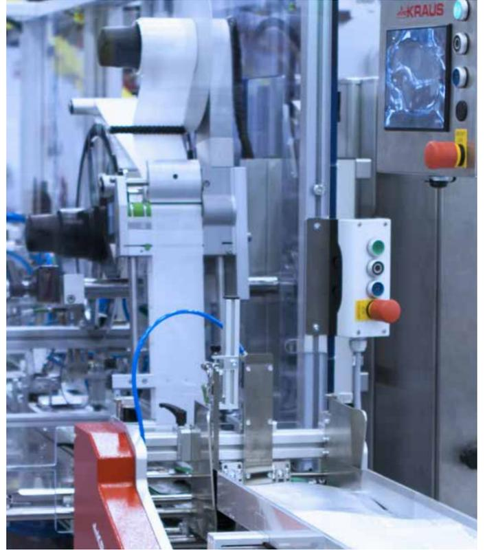
IXOR systems enable **continuous or clocked operations**. Aluminum pouches are being labeled on this picture.
