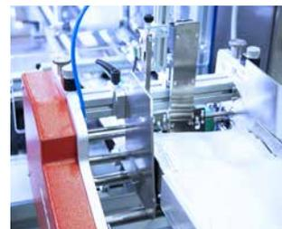
Specified machines are constructed, assembled and initially operated at the Kraus facility in Spaichingen, as well as accepted by the customers prior to delivery. In the operation at hand, Plexiglas replicas of LifePad PCR test cassettes and three-side sealed pouches are fed by friction feeders from preceding processes to a machine combined for labeling and packing.
