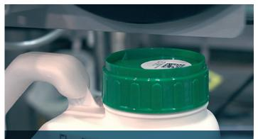
No touch with the product surface In case of recessed canister caps, labels are blown on by air jet.
