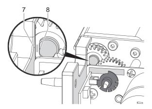
3. Turn the axle (5) of the circular blade with a screwdriver for slotted head screws (slot width 7 mm) so that the planar area (8) of the blade axle becomes parallel to the base plate (7).
