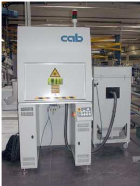
Ytterbium fiber laser system with fume extractor
