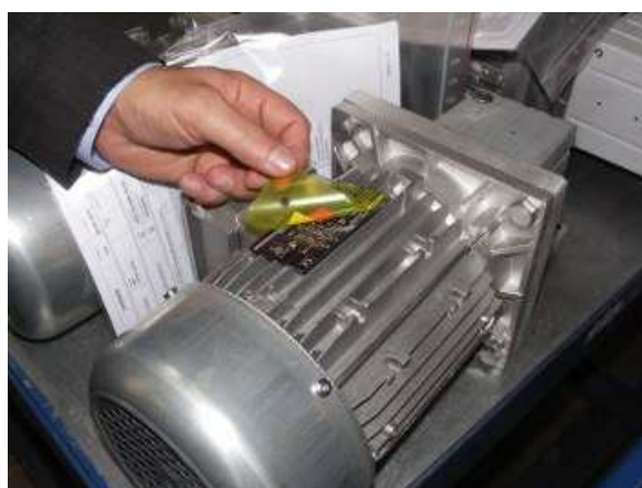
During assembly the typeplate is protected by adhesive
