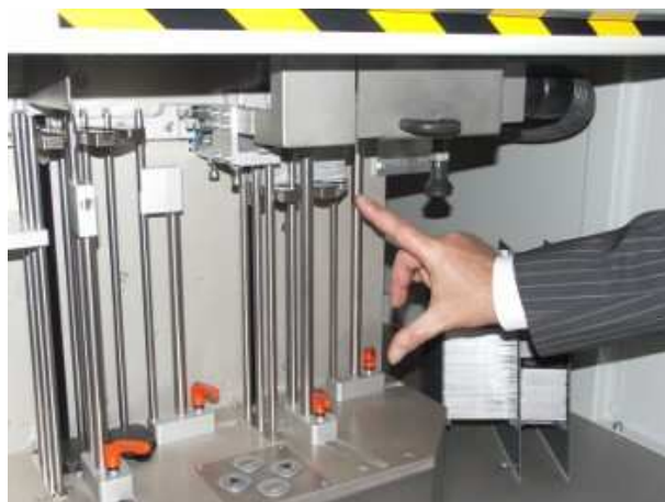
Typeplate handling module following the FIFO principle
