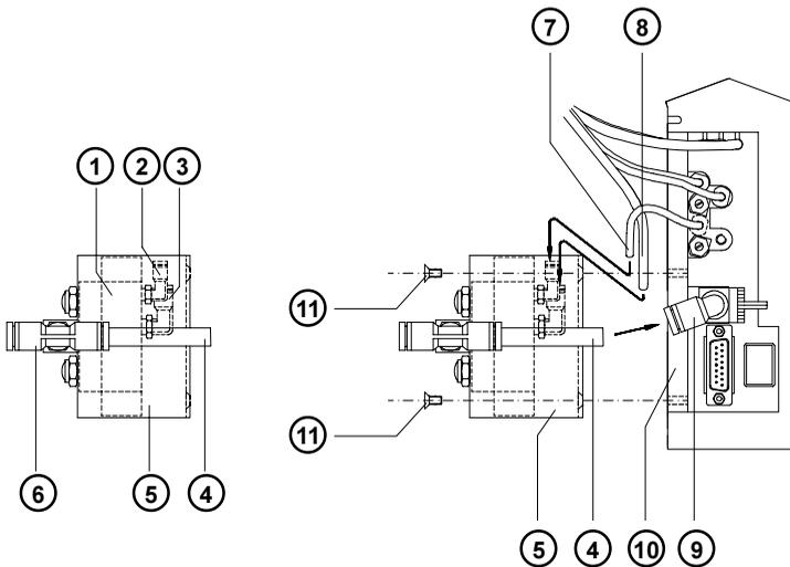
**Fig. 4a Installation of the external blow valve**
