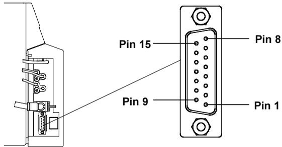
Fig. A-1 Connector of the PLC Interface
