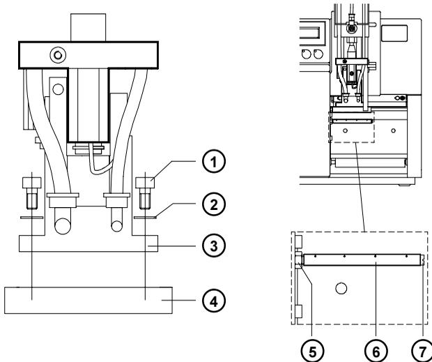
**Fig. 4d Installation of the pad and the blow tube**
