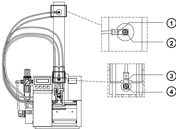
**Fig. 5.2b Throttle valves at the lift cylinder**
