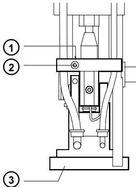
**Fig. 5.1e Adjustment of the blow-on angle of the pad**
