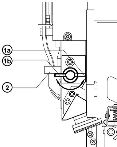
**Fig. 4c Unlocking the securing device**
