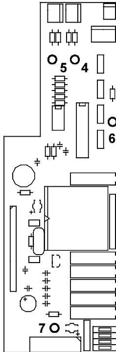
**Fig. C-2 LED on the applicator control PCB**
