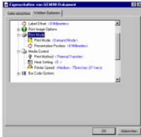
Figure 8i Printer Setup - Document Properties Window under Windows NT 4.0, 2000 and XP Section "Print Mode and Media Control "
