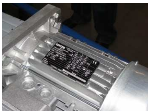
Well readable typeplate on the gear motor
