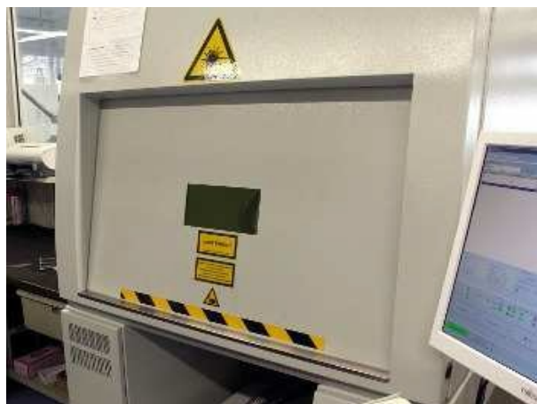
The Laser Tool Coding System enables to mark tools out of steel or hard metal with a Data Matrix Code in a few seconds
