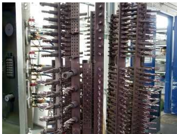
Coating the tools generally takes four to six hours. Then, the parts are passing various testing processes and are finally assigned back
