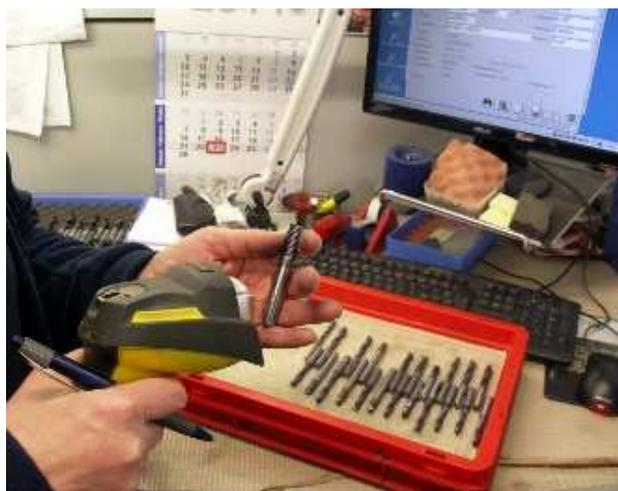
The Laser Tool Coding System enables to easily and perfectly assign the tools back to their commission number after the coating process
