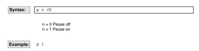
Sets the printer into pause mode, if a print job runs, it will stop after the label is printed. The Pause LED lights on the front panel.
