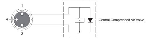
Fig. 10 Connector central compressed air valve
