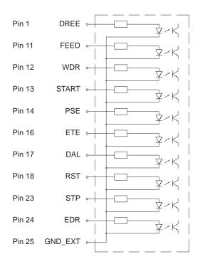
Fig. 3 Circuit of the inputs
