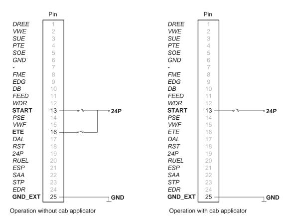
External minimum circuit of the I/O interface with external voltage supply Fig. 6
