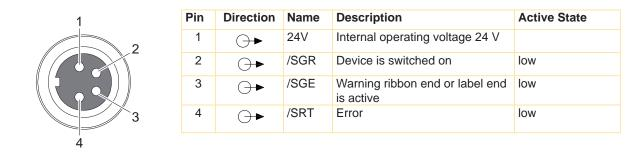
Fig. 8 Connector warning light Table 2
