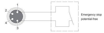
Fig. 9 Connector emergency stop
