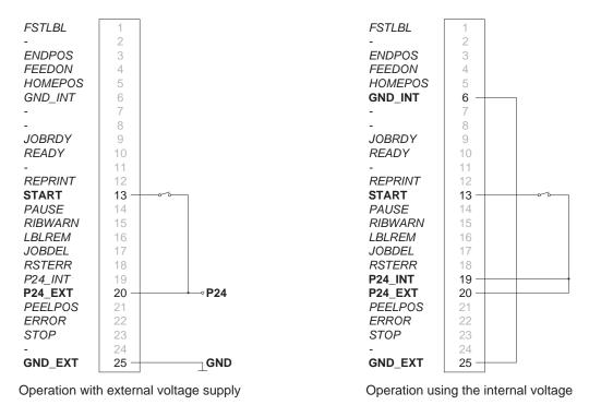
Figure 9 External circuit for peeling-off on demand without present sensor with switching signal START
