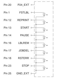
Figure 2 Connecting inputs
