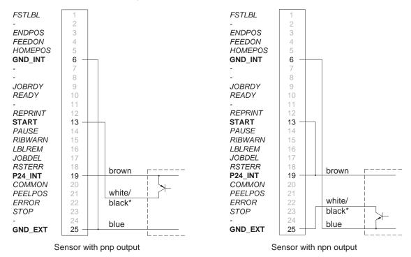
Figure 12 External circuit for releasing the signal START using optical sensors \* depending on sensor type
