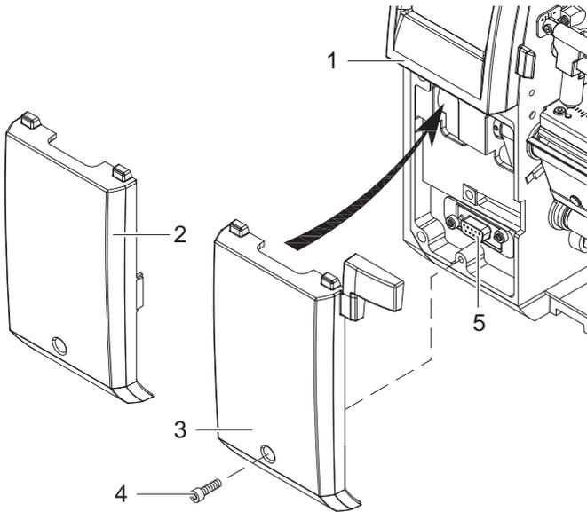
Figure 1 Mounting the present sensor
