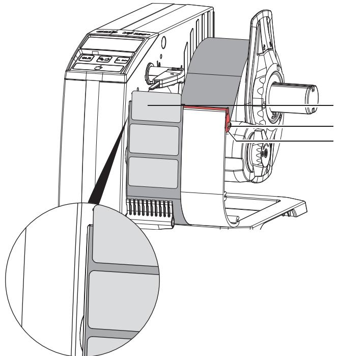
The label material must run **parallel** to the chassis.
