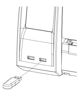
Figure 4 Inserting the service key
