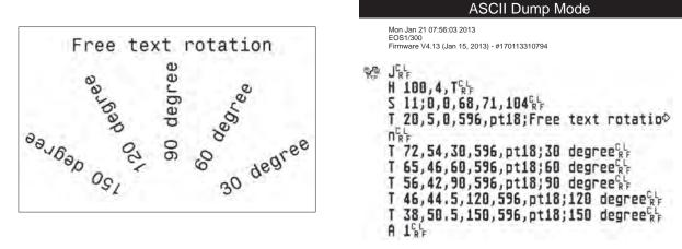
Figure 17 Example label printed normally (left) and in ASCII Dump Mode (right)
